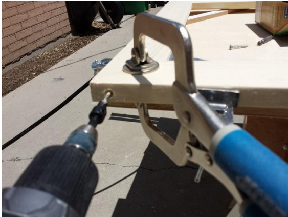
Pre-drill with countersink, then nail with 2" finish nails
