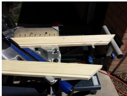
I used a stop to ensure the cuts came out the same
