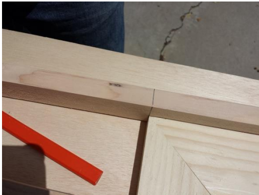
Marking where I need my miter to end
